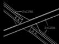
SPAN CONNECTION OF C200 BRACING WITH M20
