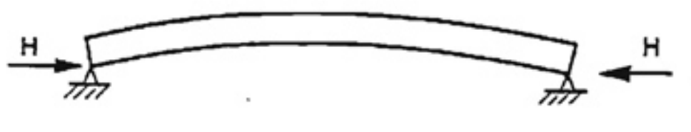
b) situation in an initial stage of the fire ( \theta_s = 20 + (\Delta\theta_s)_1 )
